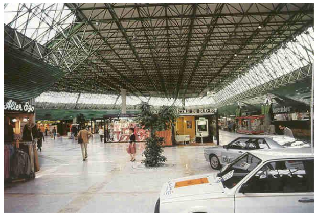
Fig.24 Example of space bar roof
